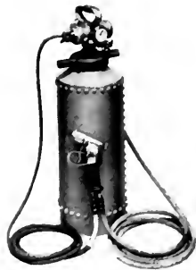
A Spray Engineering Company's outfit for painting with compressed air. The extreme simplicity of this apparatus has gained it great favor among shipyards.
